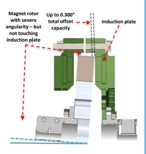
though – it's the additional load/force applied to the shafts, bearings and seals that truly does the damage. Consider the equation for bearing life ( $L_{10}$ ) above. Increasing the bearing load from misalignment has an exponential (cubic) negative effect on the lifespan of the bearing. Based on this equation, misalignment forces that double the total load on the bearing will result in an eight times reduction in bearing life!
